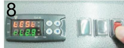
Put Power On. The Green number displayed is the programmed operating temperature (°C) and the Red is the current temperature.
