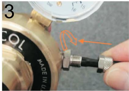
Tighten nut with spanner
