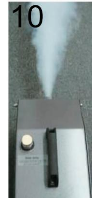
To make smoke press the Black Smoke Switch to On (1). 3-4 seconds later smoke production will start.
