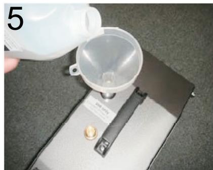
Remove filler cap and slowly add smoke oil to the Phantom. Check the sight glass and **do not overfill**. If an airlock is seen in the sightglass simply rock the machine gently forward and backward until it has cleared.
