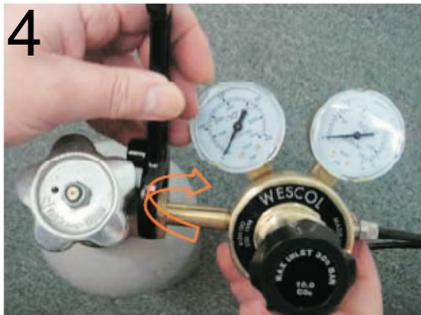
Attach regulator to CO2 cylinder and tighten with spanner supplied
