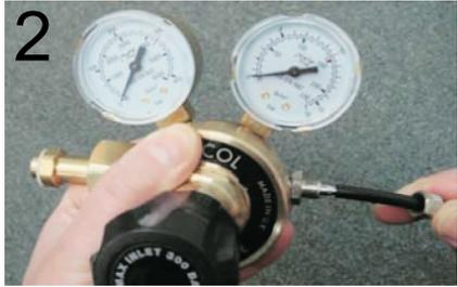
Push Gas hose onto regulator as shown
