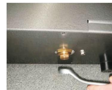
If sending the machine via a courier we always recommend oil is removed from the machine to prevent spillage, and a drain is fitted to assist this
