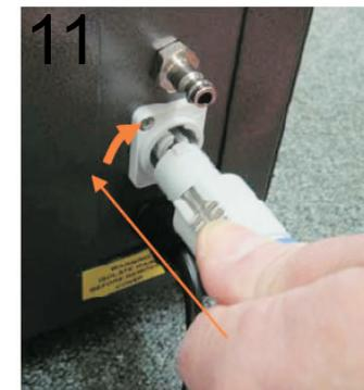
To use remote push in an twist to the right The remote switch then duplicates the function of the Black Smoke Switch on the machine. If either switch is on, the Phantom will produce smoke. To remove pull back on the metal latch, twist to the left and pull out
